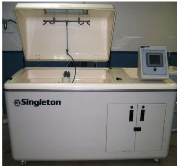
Photograph 5 Cyclic Corrosion Test Chamber
