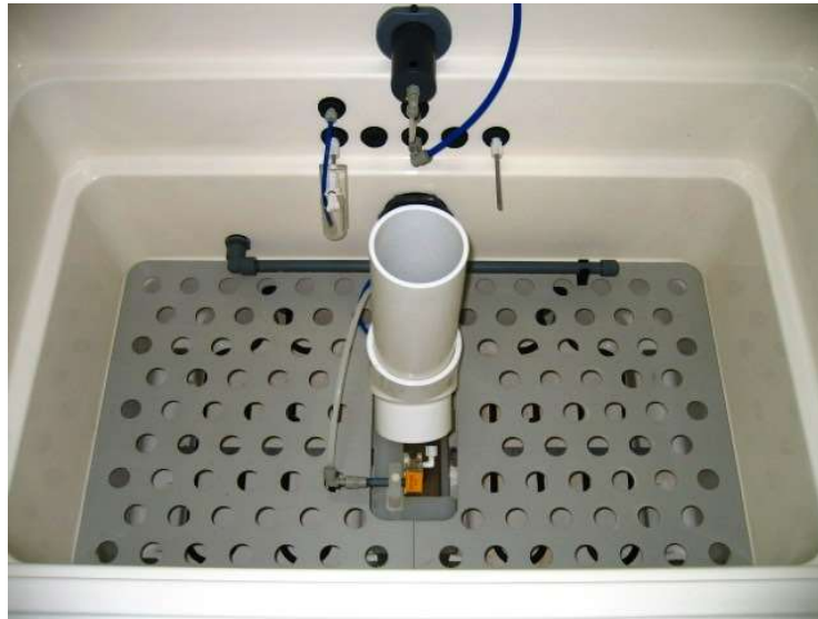
Photograph 6 Cyclic Corrosion Test Chamber
