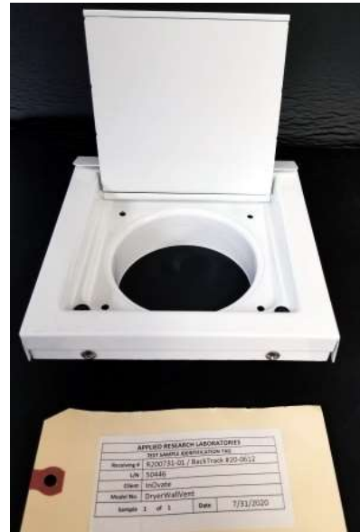
Photograph 2 DryerWallVent (Unexposed) ARL Sample ID #20-0612
