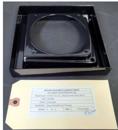
Photograph 10 DryerWallVent Frame (Exposed) ARL Sample ID #20-0613
